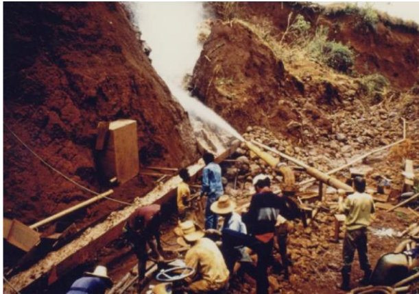
Figure 17. Hydraulic platinum mining from laterite (Yubdo, western Ethiopia)
