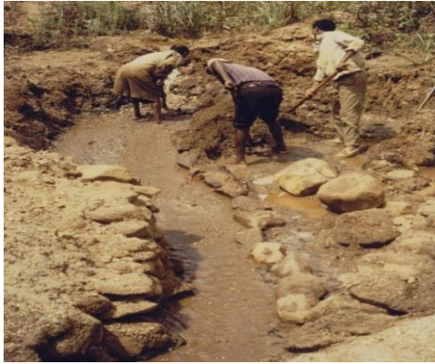
Figure 13. Ground sluicing for placer gold Adola, southern Ethiopia
