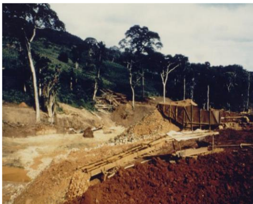
Figure 18. Hydraulic mining of placer gold (Adola area, southern Ethiopia)
