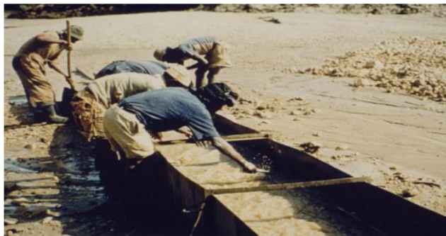
Figure 20. A sluice box used in placer mining to recover gold, Adola, southern Ethiopia.
