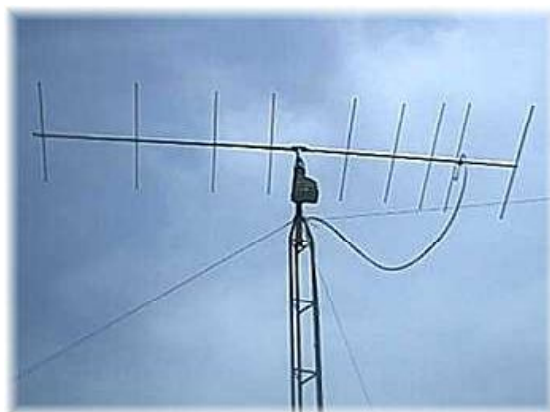
Fig 3.24 Yagi Uda Antenna
