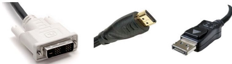
Fig. 5.8 Connectors of different digital display interfaces. From left to right: DVI, HDMI, DisplayPort
