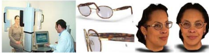
Fig. 18. Example of 3D virtual-make-over. Left: 3D acquisition system 3D iView of Visionix Ltd. (Israel). Center: 3D model of frame and lenses. Right: virtually placed eyewear onto a 3D face model.
