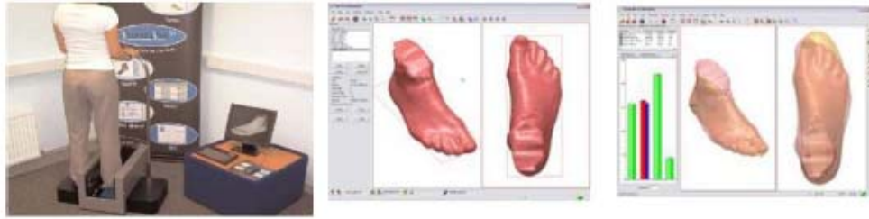
Fig. 23. Made-to-measure for footwear. Left: 3D foot scanner Shoemaster of CSM3D International Ltd. (UK). Center: 3D model of the scanned foot. Right: software solution for the design of made-to-measure shoes.
