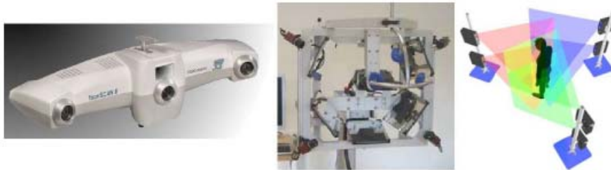
Fig. 8. White light projection systems. Left: face scanner faceSCAN-II of Breuckmann GmbH (Germany), with two cameras and one projector. Center: face scanner Gscan of IVB GmbH (Germany), with one projector, five cameras and mirrors system. Right: full body scanner Mega 3P of InSpeck Inc. (Canada) with six units, each with a camera and a projector.
