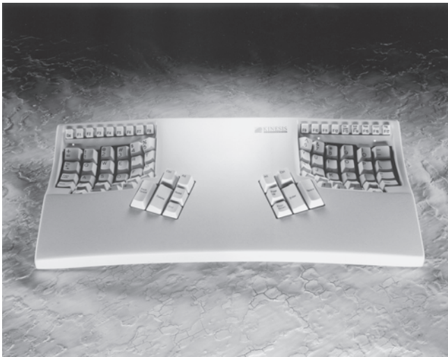
Figure 5.11 Separate banks of keys for each hand may relieve wrist strain. (Photograph kindly supplied by Kinesis Corporation, Bellevue, Washington, USA.)
