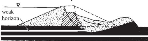
(f) Instability (3): failure of downstream foundation due to overstress of soft, weak horizons
