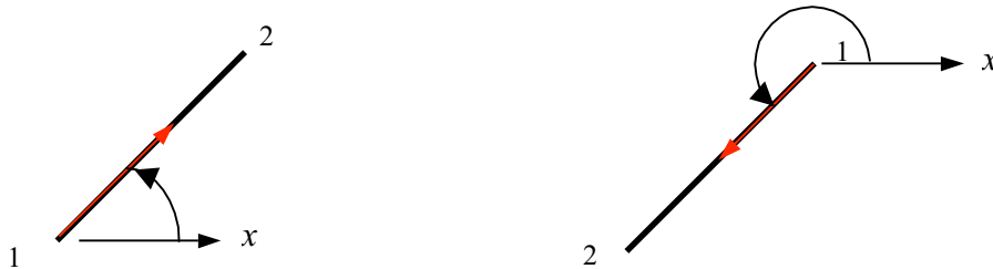
Member direction is defined from the starting node to the end node.
