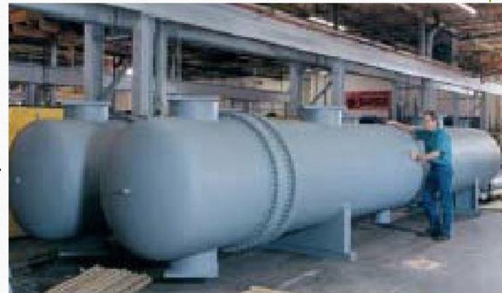
Fig. 1.1: shell and tube heat exchanger
