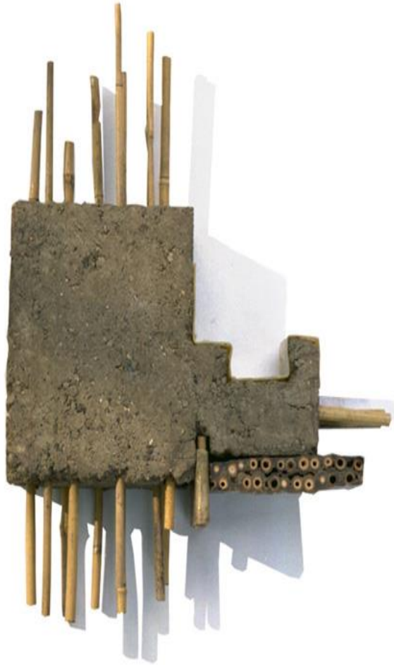
Traditional Earth Reinforcement
