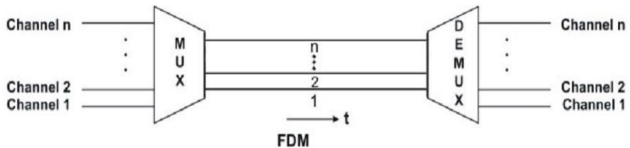
Figure 2.7.2 Basic concept of FDM
