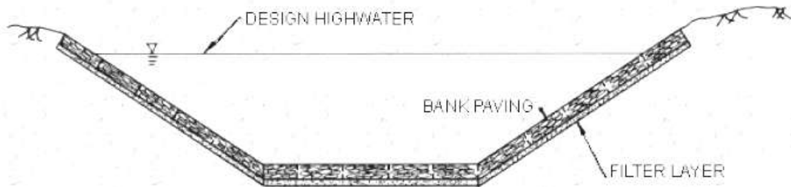
Figure 5.14 Rock and Wire Mattress Installation Covering the Entire Channel Perimeter
