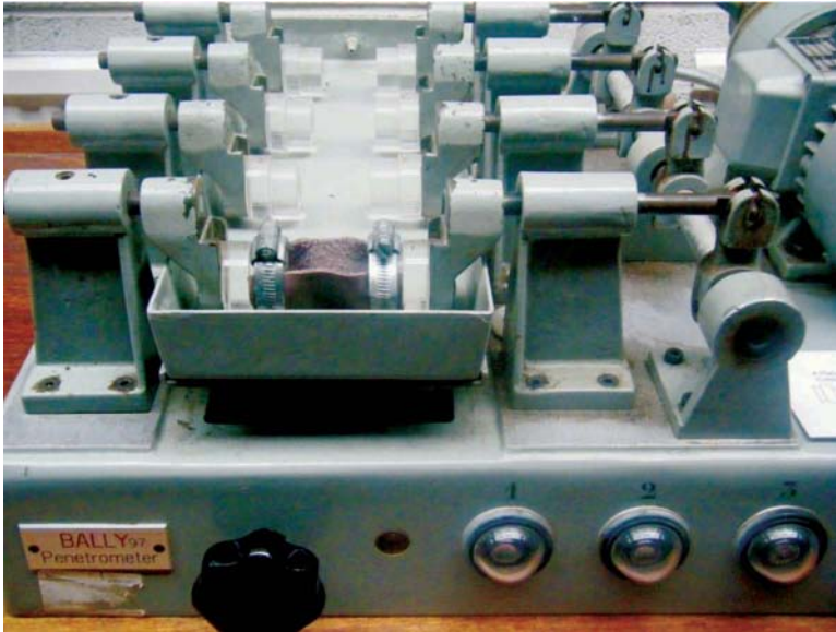
Figure 17.18 Bally Penetrometer for measuring water resistance: bent leather is flexed in a bath of water until penetration through the cross section occurs.
